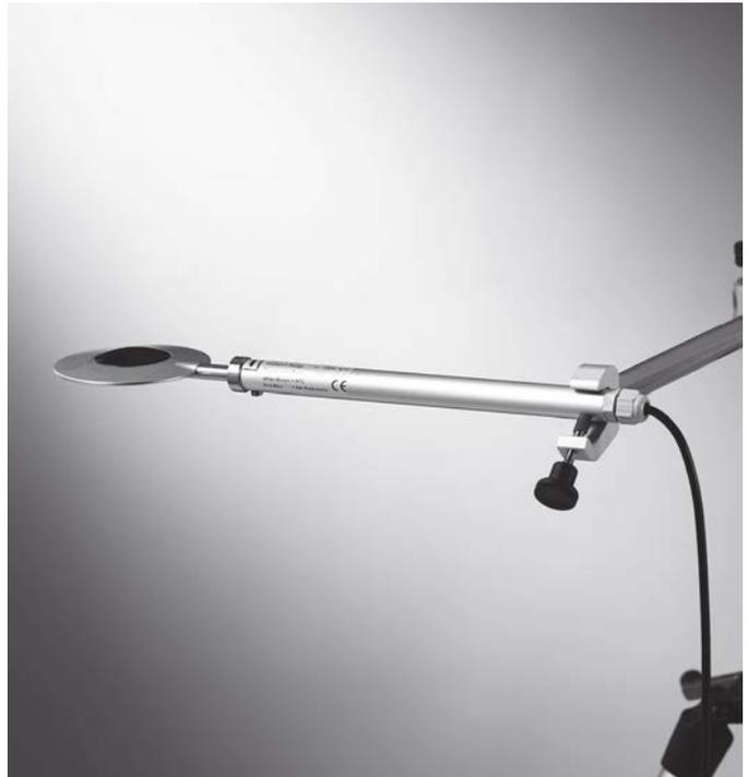
The face of the probe marked by the symbol
