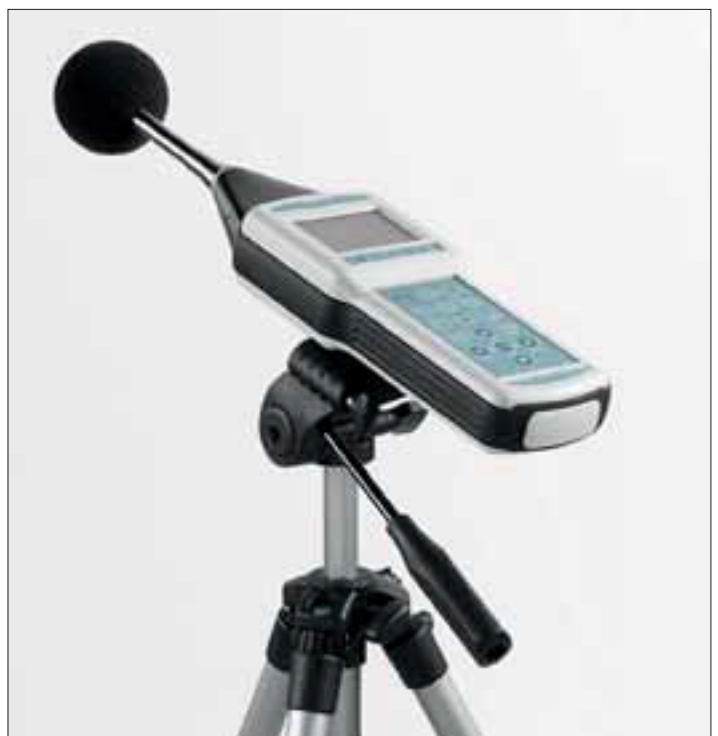
Noise Studio: NS5 "Environmental Noise" module; sound sources analysis with tonality and impulsiveness evaluation.
