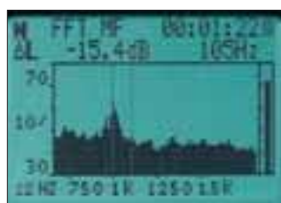
FFT narrow band spectrum (option HD2110.06)
